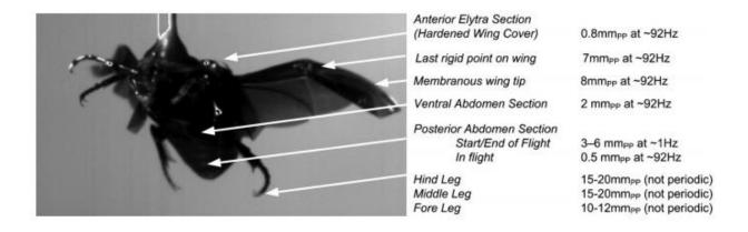
4.7 The figure shows measured frequencies and amplitudes of vibration from a Green June Beetle. Estimate the power that could be harvested from the bug assuming a vibration amplitude of 1mm, frequency of 92Hz, mass of 0.13gram (10% of the beetle's mass), and damping  $\zeta = 0.1$
