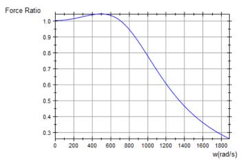
Now the measurement slightly over-estimates the force, before dropping off. We can maximize the frequency range by allowing the maximum value of the force ratio to just hit 5% error. We need to first solve for the frequency at which the max occurs (differentiate, set to zero and solve – use mupad)
